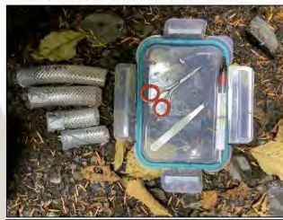
Sample (fin clip) collection kit showing restraint tubes, scissors, forceps, and thermometer.
